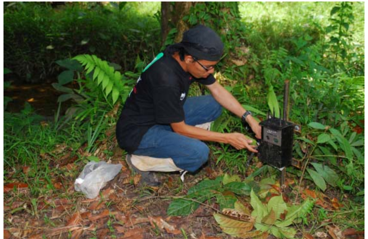
Azlan Mohamed setting up a camera-trap in Deramakot Forest Reserve. The cameras are kept in steel housings with sharp nails on top to protect them from damages by elephants (Photo K. Povey).
